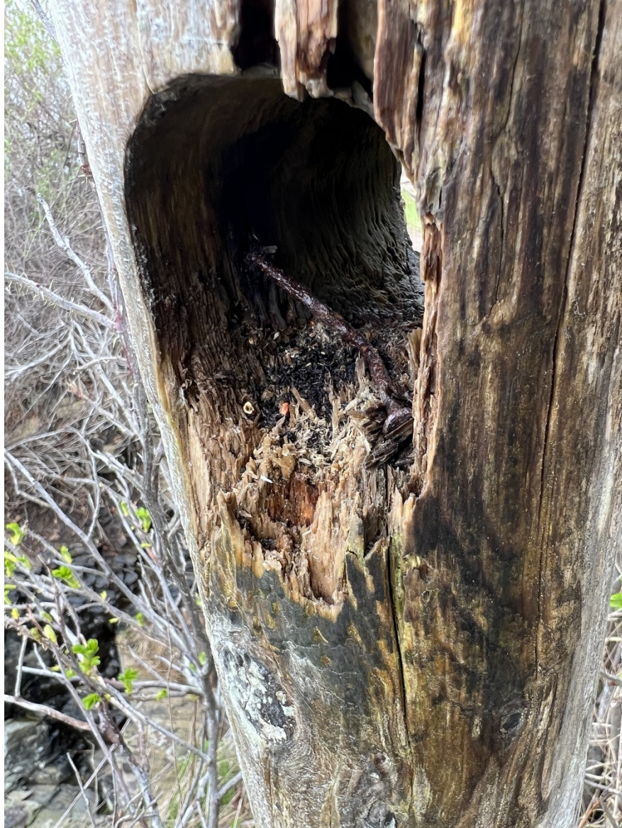
Figure 6. Photograph of rotten fence post taken by counsel. (A285).
